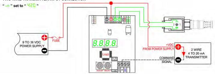
**PLEASE NOTE:** For "0 to 5 VDC" & "0 to 10 VDC" command input drivers, it is recommended to use independent negative conductors for power supply and analogue output channel (PLC/PC) to maintain command signal accuracy due to voltage drop on long cable runs.
