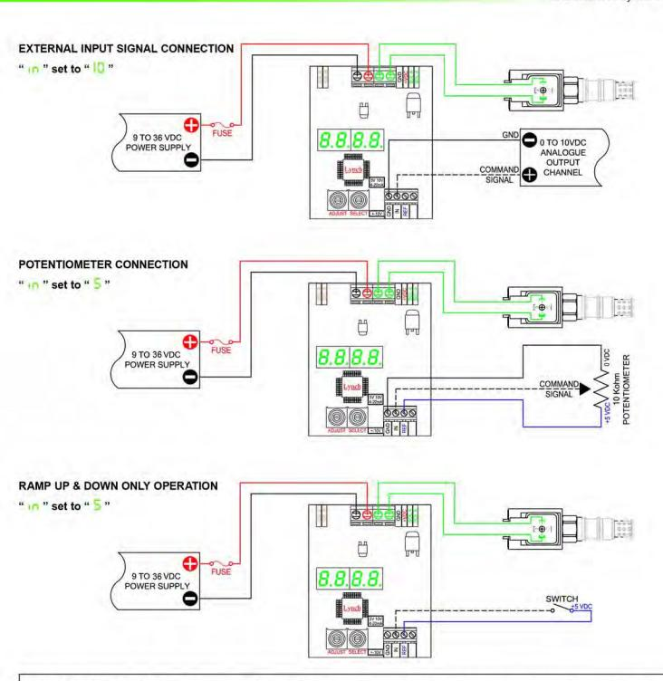
**PLEASE NOTE:** For "0 to 5 VDC" & "0 to 10 VDC" command input drivers, it is recommended to use independent negative conductors for power supply and analogue output channel (PLC/PC) to maintain command signal accuracy due to voltage drop on long cable runs.
